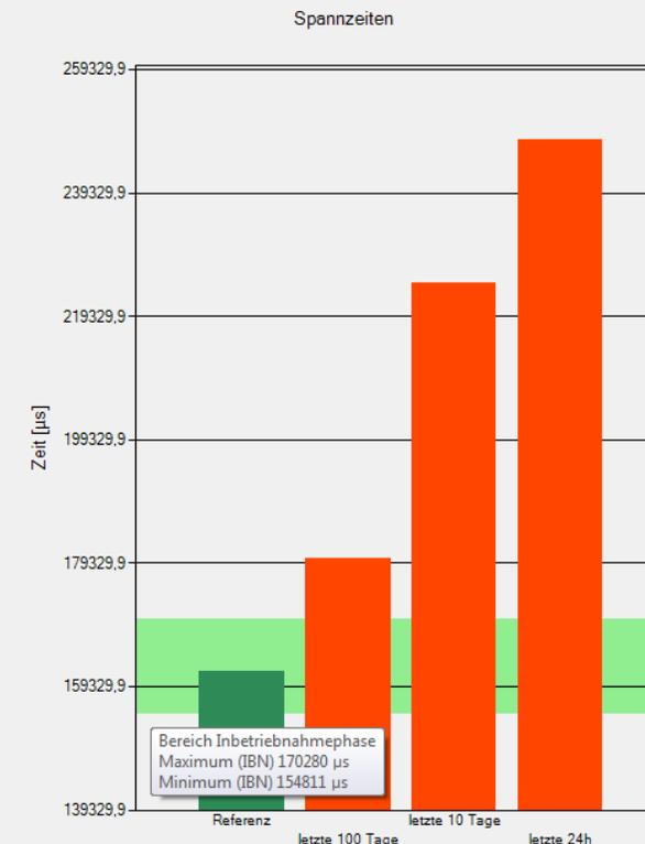
Slowly increase of clamping time → damage process or wear of clamping system parts
