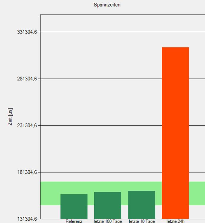
Fast increase of clamping time → broken spring of the clamping system
