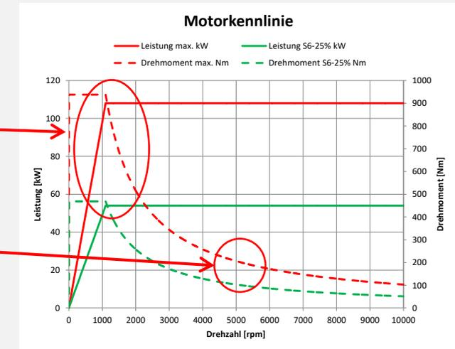
Conclusions can be drawn about the load of the spindle bearing and the thermal load of the motor from the running time of the spindle with respect to predefined speed ranges and torque ranges.
