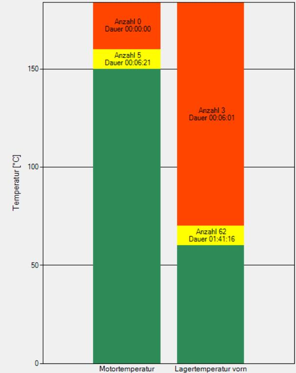
Violations of the temperature warning limit → possible failure process at the bearing
