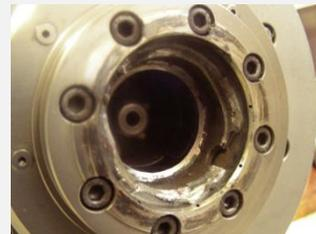
**Damaged tool interface**
