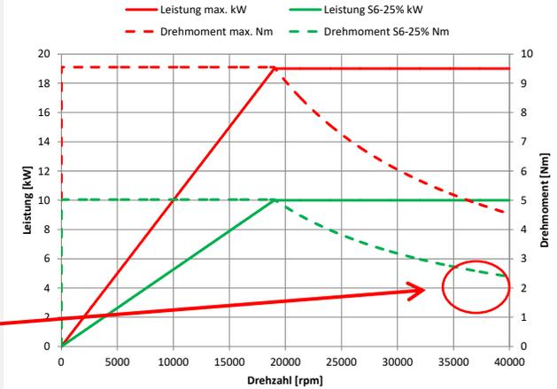
Mainly operation at high speed → Possible damage process at the grease lubricated bearings
