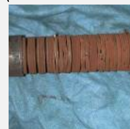
Broken spring of clamping unit
