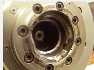
Damaged tool interface
